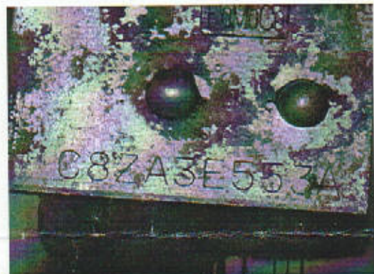
Fig 2) Marking on original relay.
