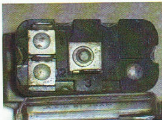
Fig 3) Terminal numbering- original relay.
